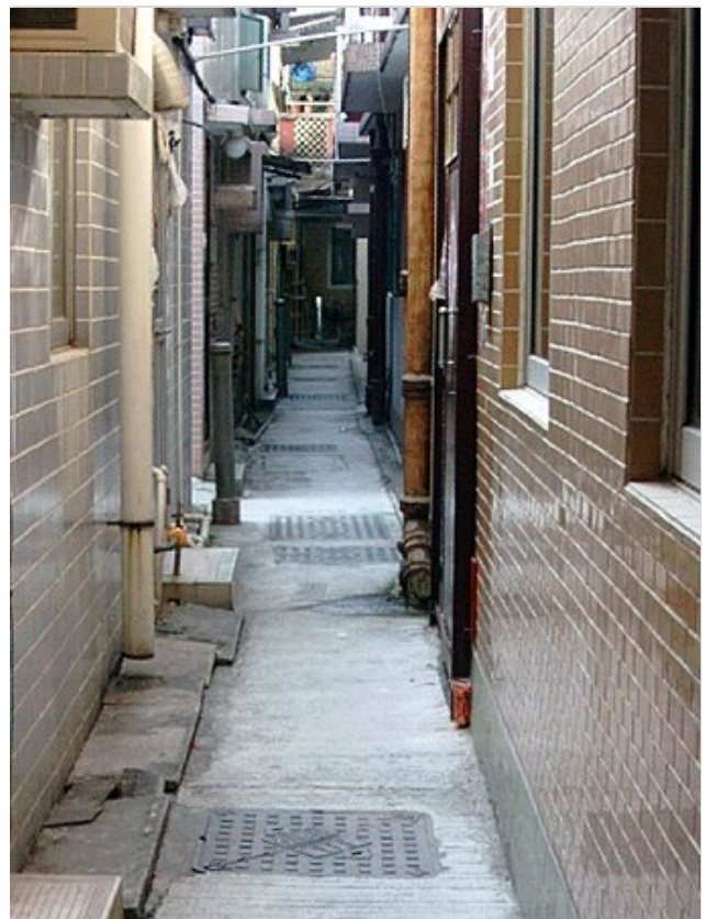
Narrow Streets unsuitable for conventional gravity sewerage system
